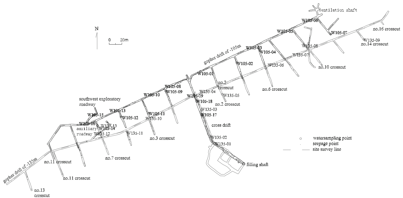
Fig. 4 Sketch of hydrogeological survey in -105, -135 m level
